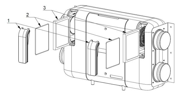
CAUTION: When replacing the filters, make sure the arrow points in a direction compatible with the air flow.
