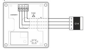
The setting of jumper links No. 1 and No. 2 defines the VSHC sensor address in C14 network. The sensors can have numbers from 6 to 9.
