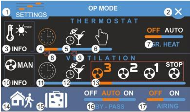
Moves to the thermostat and ventilation settings. See the SETTINGS section for a detailed description.
