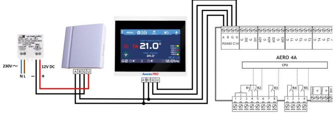
Note! Only one VACS-1 or VSPM sensor can be connected to the device.
